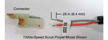
7. Connect the extension harness to the cut wires using butt-splices as shown per model type.
