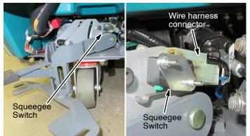
6. Cut wires close to connector and strip as shown.
